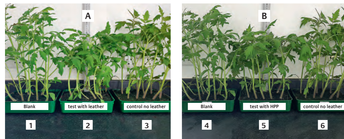
Fig.2. Plant growth after 28 days in compost containing (A) FOC leather without LEVOTAN® HPP; (B) FOC leather with LEVOTAN® HPP. Comparison with blank and control without leather.
